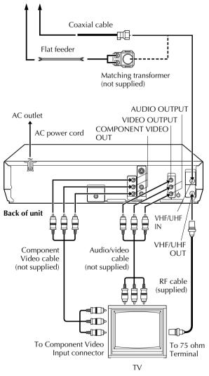
■ To connect to a TV with component video input connectors . . .
